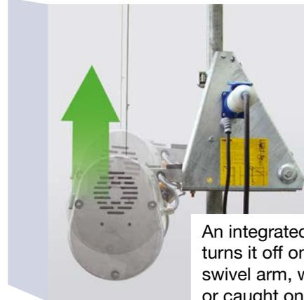
An integrated limit switch turns it off on reaching the swivel arm, when overloaded or caught on the scaffold.
