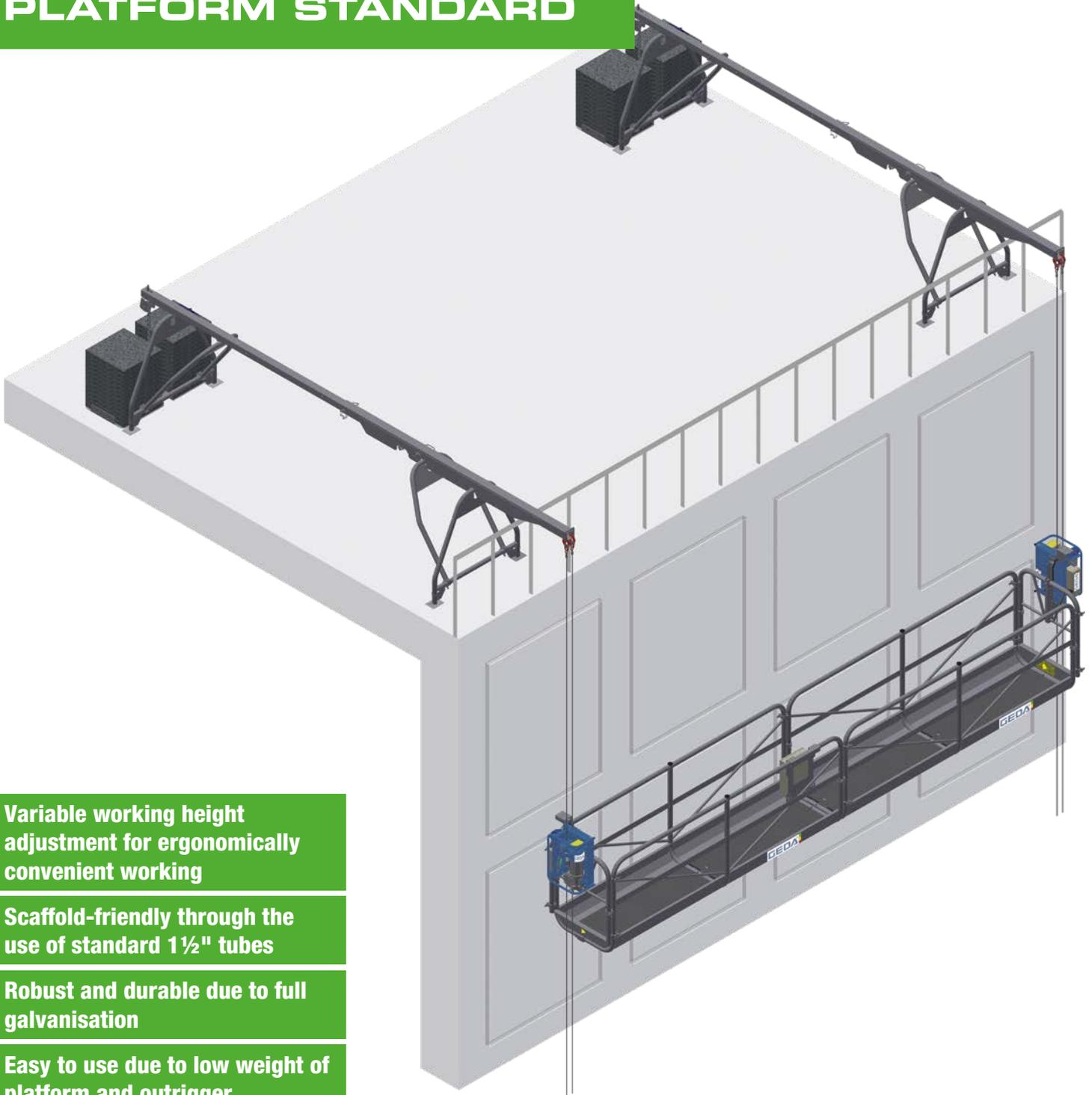
**Variable working height adjustment for ergonomically convenient working**
