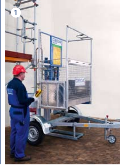
1 Automatic unloading from the trailer.
